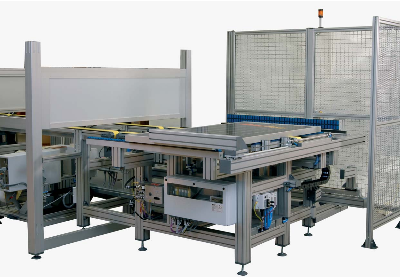
Automatic lift from horizontal to vertical transport
