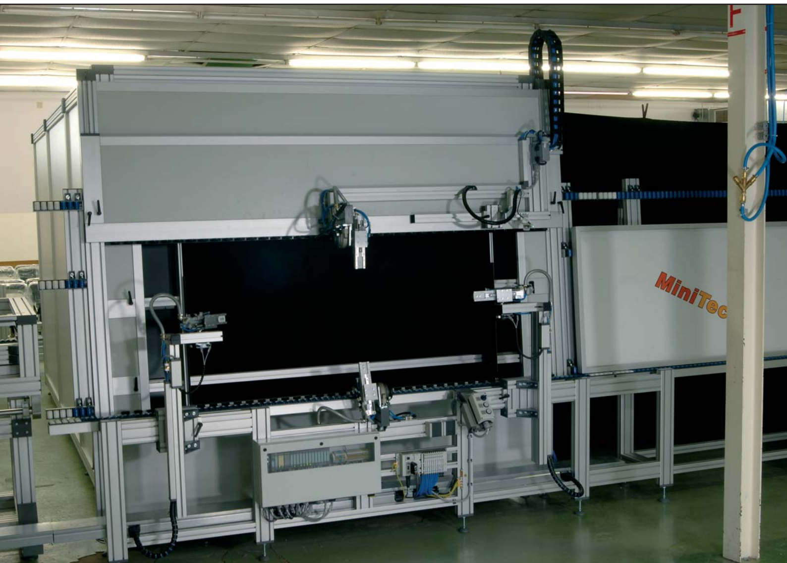
Modul flasher with integrated HV-test/isolation test
