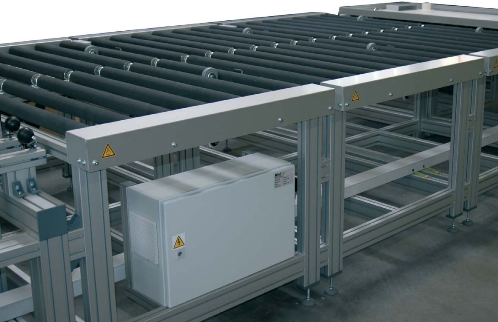
Roller conveyor with mechanical accumulation protection
