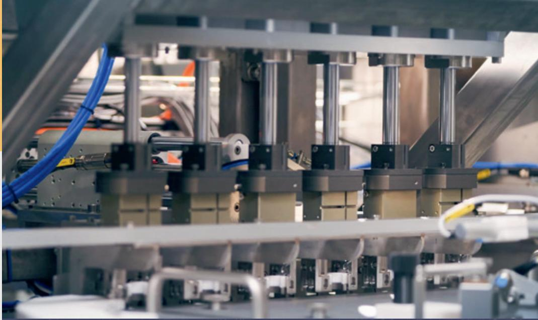
Torque and force sensors enable precise and recordable closing operations, as often required in the pharmaceutical or medical industries.
