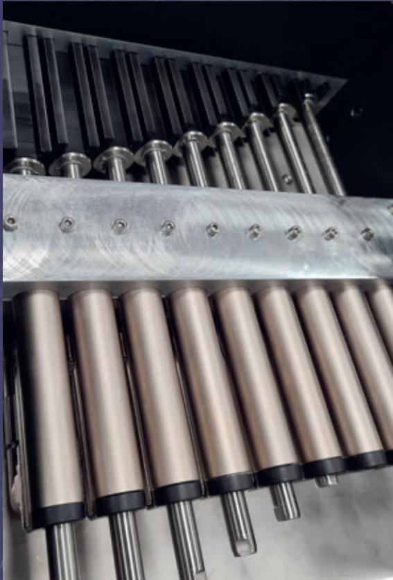
The capabilities of SYSCONA’s brand-new ProfiCurve deflector open up a whole new world of possibilities in the construction of conveyor systems. SYSCONA uses 25 mm wide high performance linear drives from LinMot’s P01 series with a stroke of 100 mm.
