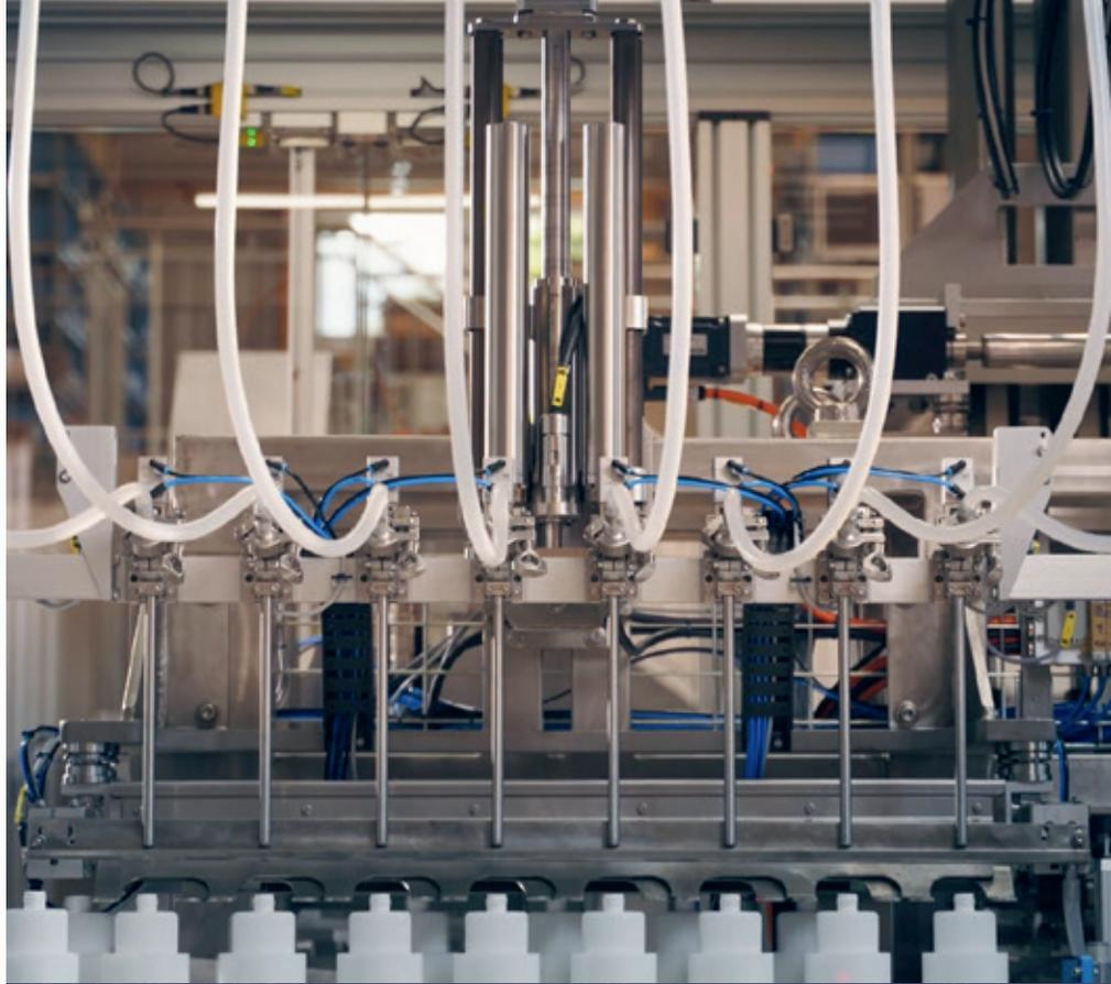
The LinMot SM01 and SM02 guides are manufactured from 316L stainless steel, which is recognised as the standard in the food, pharmaceutical and chemical industries. This is particularly important in filling systems where strict hygiene standards are essential.
