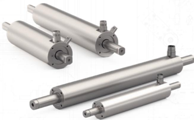
All linear motors are fitted with temperature monitoring sensors which transmit data to the servo drive. The data can be analysed in the PLC so that the motor can be kept within a constant temperature range depending on the process (e.g. food products such as fish). For some motor types, LinMot offers an optional integrated water cooling system, which leads to higher performance and lower surface temperatures. ■
